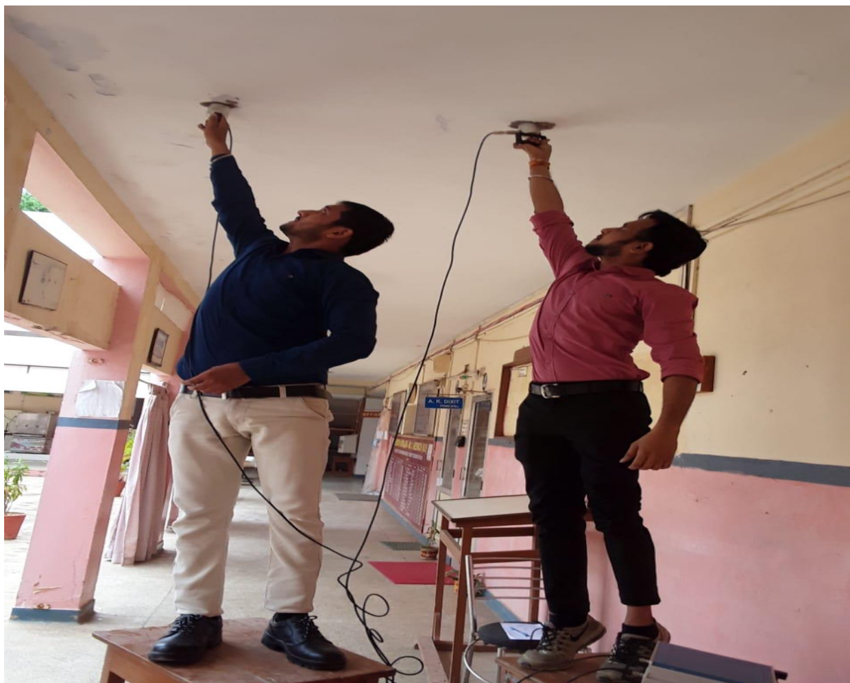
Figure 24: Rebound Hammer Testing of slab
