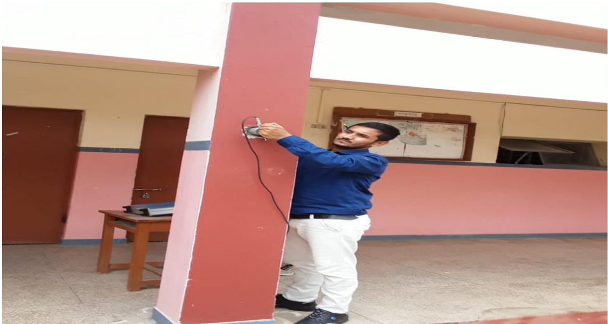
Figure 23: Ultrasonic pulse velocity Testing of column
