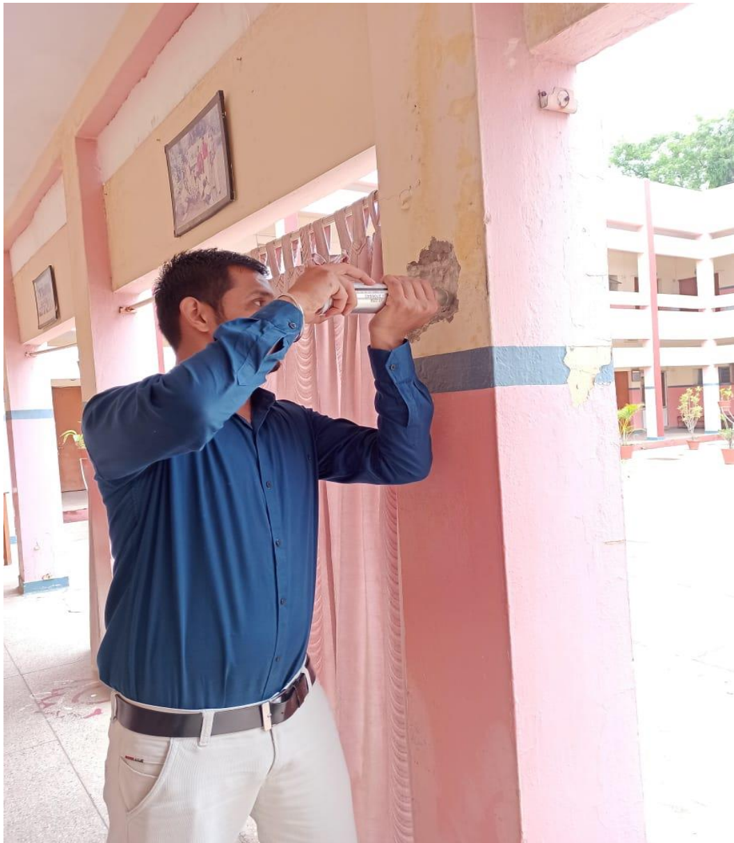
Figure 22: Rebound Hammer Testing
